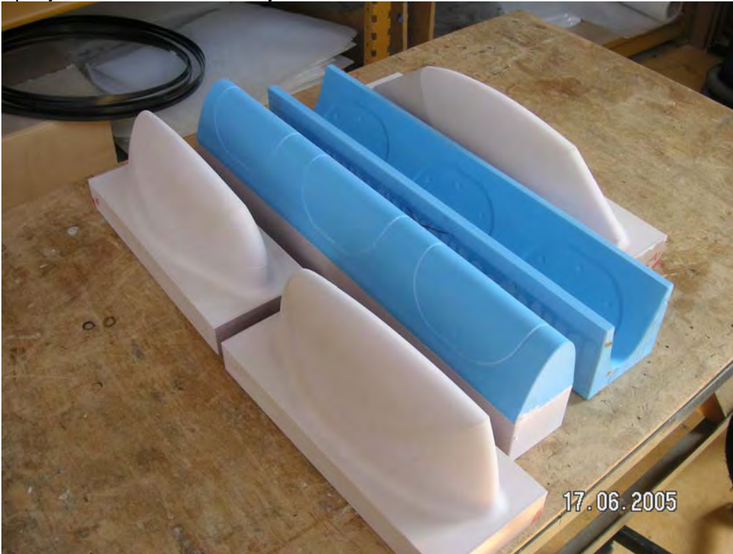
Epoxy board AB135 blue, Polyurethane board AB40 brown
