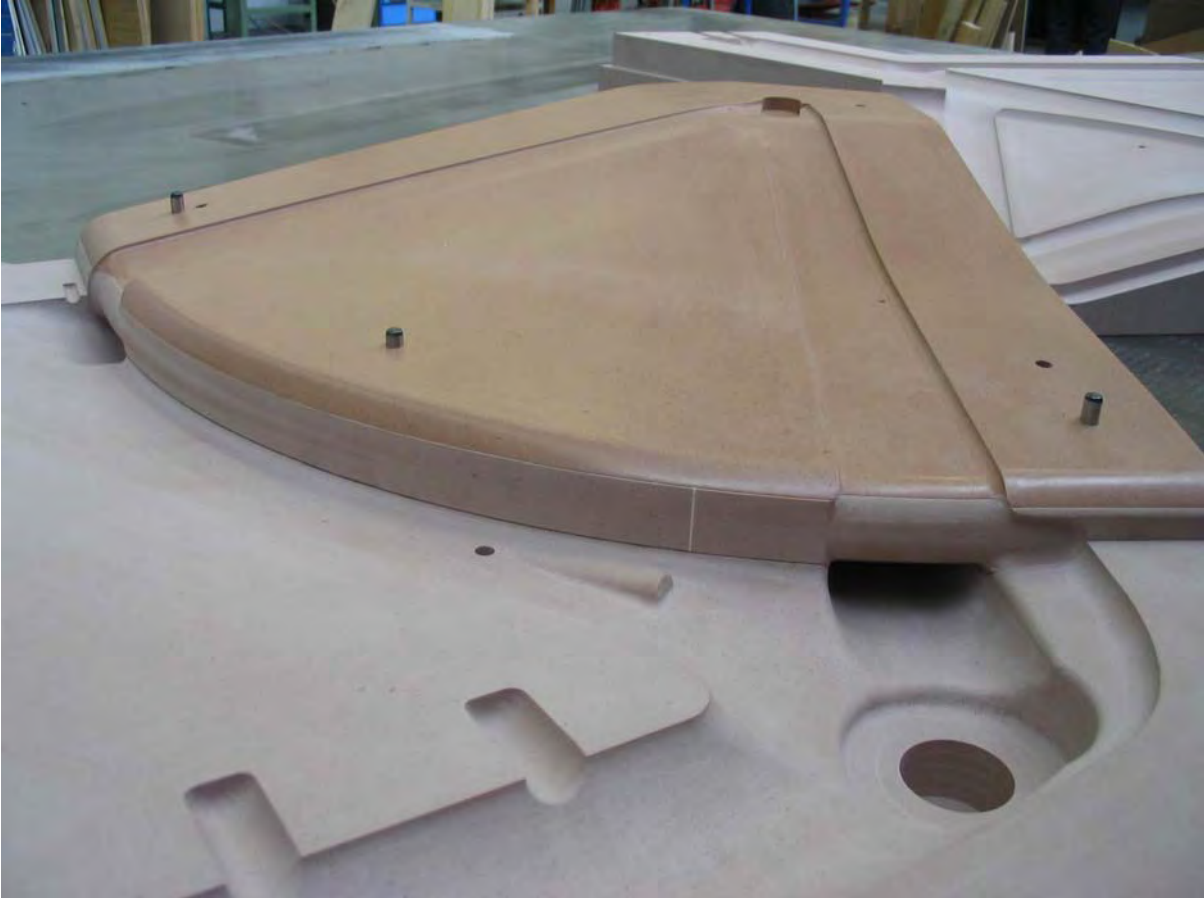
Master tool Epoxy board AB70 for the BMC time machine TT01 bicycle frame.
