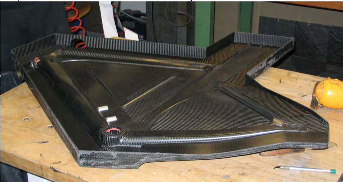
Composite tool for the BMC time machine TT01 bicycle frame
