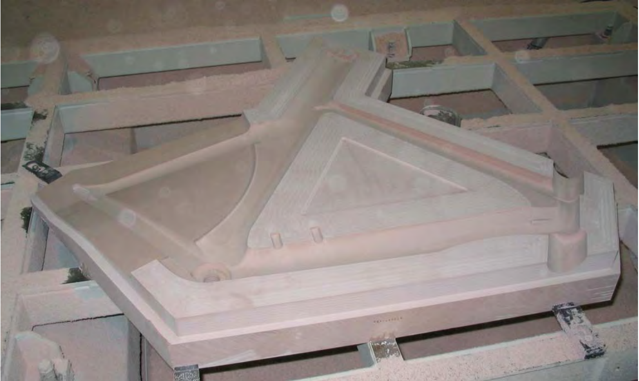
Master tool Epoxy board AB70 for the BMC time machine TT01 bicycle frame.
