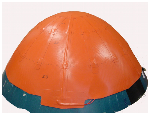
Left: a radome with 4 large areas; Right: A long heating blanket designed with 4 zones for helicopter blade repair
