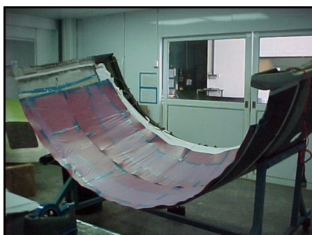
Left: a large surface of a transcowl covered by a 4 zone heating blanket Right: a complete ring abrasable silicone liner covered by a blanket. here 4 zones are differentiated and the ANITA 4Z controls the temperature of each zone
